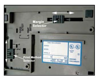
Figure 2-17. Auto-Sync Time Clock Printer Adjustment.
